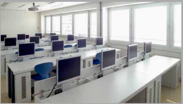
The IT version is one of the special designs of lowerable superstructures available from Elabo: TFT monitors disappear in space-saving fashion into the body of the lowering assembly. In addition there is room for a keyboard and mouse.
