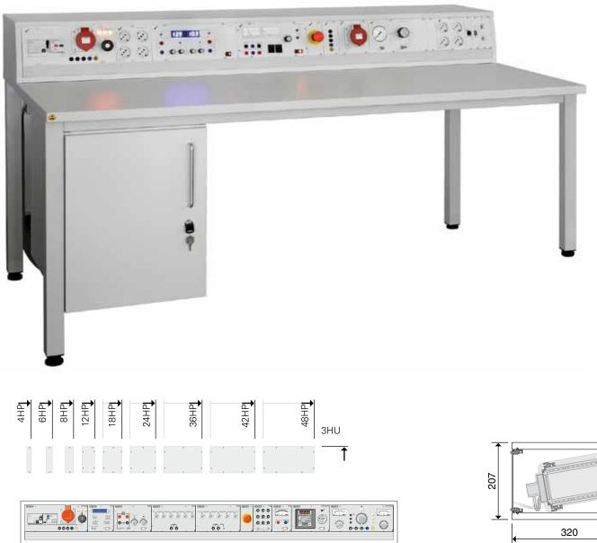
The aluminium profile frame used on the desktop rack is constructed like a rack mount. The front and rear transverse profiles have punch holes and M 2.5 threads in a 5.08 mm grid in order to hold guide rails, built-in components and connectors in accordance with the standard. The network supply for the built-in component points comes from a standardised connector.
